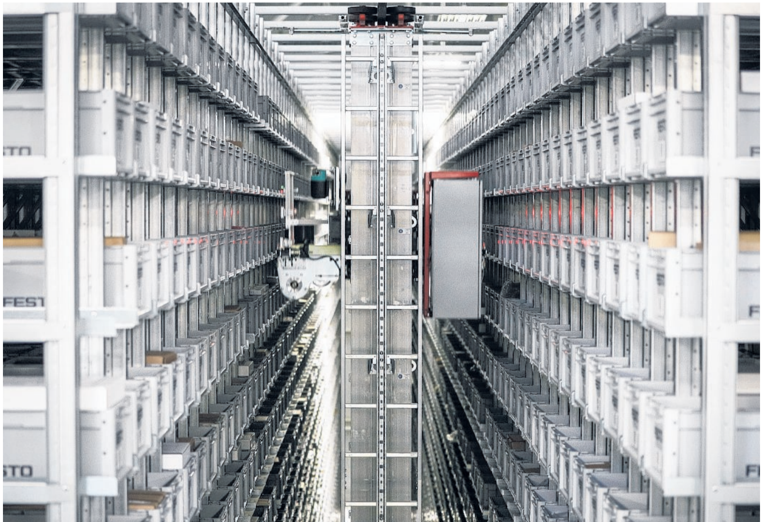
A robotic distribution system uses laser guides to move through stacks. CEOs suggest there will be a high take-up of automation.
