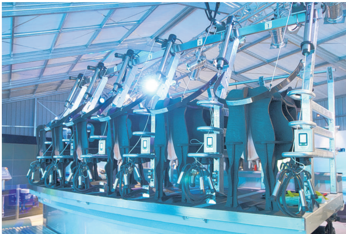
The Centrus 84 Rotary Platform easily handles a herd of more than 3000 cows, milked three times a day.
